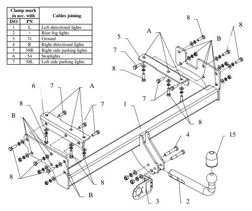
This towing hitch is designed to assembly in following cars: **MITSUBISHI OUTLANDER**, produced since 04.2003 till 03.2007, catalogue no. **Z31** and is prepared to tow trailers max total weight **1500** kg and max vertical load **75** kg.
