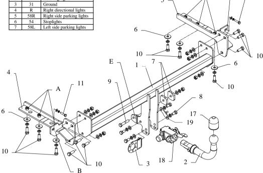
This towbar is designed to assembly in following cars: HONDA FR-V produced since 2005, catalogue no. Y31A and is prepared to tow trailers max total weight 1500 kg and max vertical load 90 kg.
