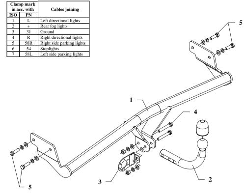
This towbar is designed to assembly in following cars: **KIA RIO, 5 doors,** produced since 09.2005 till 09.2009, catalogue no. **T50** and is prepared to tow trailers max total weight **1100 kg** and max vertical load **50 kg**.
