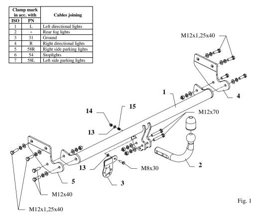
This towbar is designed to assembly in following cars: **KIA RIO, 4 doors,** produced since 2005 till 2008, catalogue no. **T48** and is prepared to tow trailers max total weight **1100 kg** and max vertical load **50 kg**.
