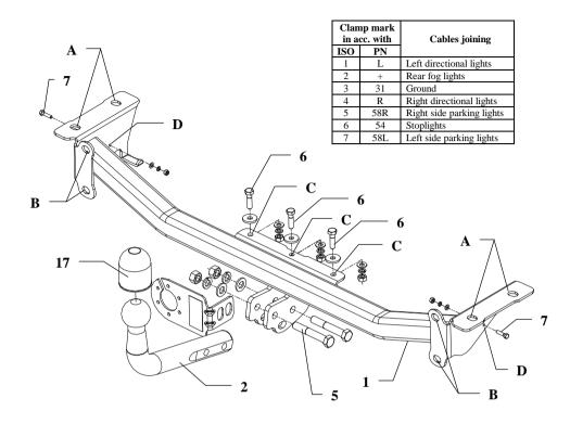
This towbar is designed to assembly in following car: **FIAT CINQUECENTO**, catalogue no. **S07**, produced since 1992 till 1998 and is prepared to tow trailers max total weight **400 kg** and max vertical load **28 kg**.
