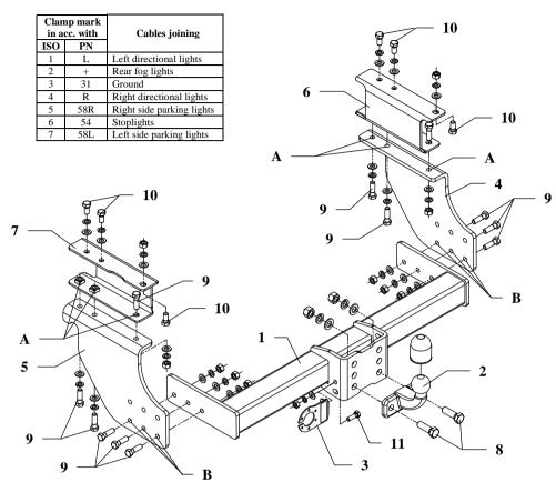
This towing hitch is designed to assembly in following cars: **FIAT IVECO DAILY 35C/50C, metal built-up, loading platform, with step,** produced since 05.1999 till 12.2013, catalogue no. **R29** and is prepared to tow trailers max total weight up to **3500 kg** and max vertical mass **100 kg**.
