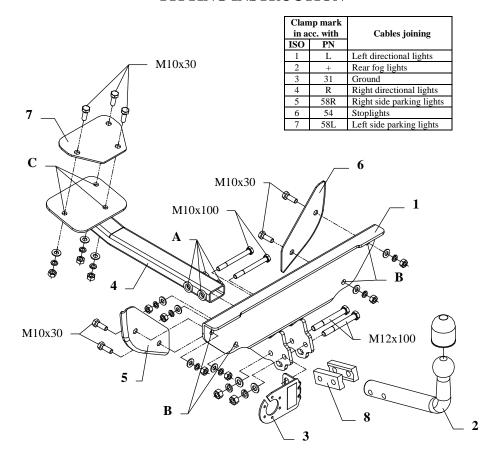
This towbar is designed to assembly in following cars: **FIAT PUNTO, 3-5 doors,** produced since 1994 till 08.1999, catalogue no. **R07** and is prepared to tow trailers max total weight **1300 kg** and max vertical load **50 kg**.
