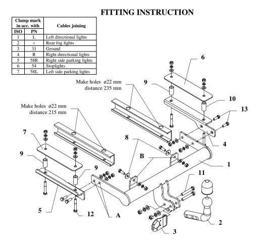
This towbar is designed to assembly in following car: CITROEN SAXO 3-5 doors, produced since 1996 till 2004, catalogue no. P09 and is prepared to tow trailers max total weight 1100kg and max vertical load 50 kg.
