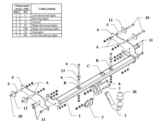
This towing hitch is designed to assembly in following car: **CITROEN C15**, produced since 1985 till 2007, catalogue no. **P06** and is prepared to tow trailers max total weight **900 kg** and max vertical load **45 kg**.
