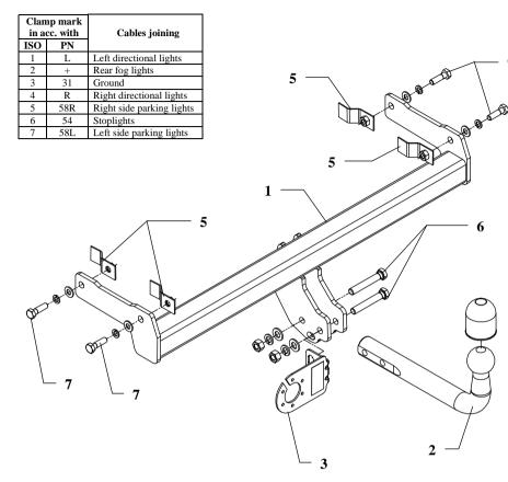
This towbar is designed to assembly in following cars: SKODA FELICIA PICK-UP and VOLKSWAGEN CADDY PICK-UP, both produced since 1996, catalogue no. H11 and is prepared to tow trailers max total weight 1000 kg and max vertical mass 50 kg.
