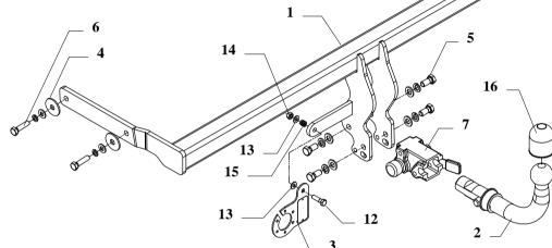
This towbar is designed to assembly in following car: **RENAULT MEGANE 4 doors,** produced since 2003, catalogue no. **G43A** and is prepared to tow trailers max total weight **1300 kg** and max vertical load **75kg**.
