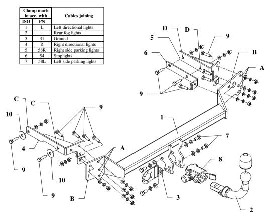
This towbar is designed to assembly in following car: **RENAULT CLIO B and C, 3/5 doors**, produced since 03.1998 till 09.2005 and **CLIO CAMPUS 3/5 doors**, produced since 2005 till 2010, catalogue no. **G29A** and is prepared to tow trailers max total weight **1200 kg** and max vertical mass **75 kg**.
