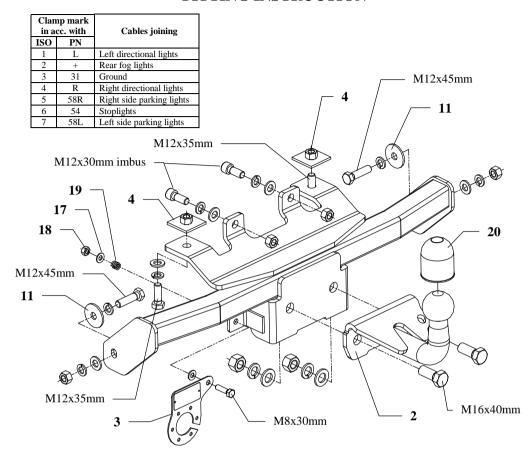
This towing hitch is designed to assembly in following car: **RENAULT ESPACE** produced since 11.1996 till 10.2002, catalogue no. **G26** and is prepared to tow trailers max total weight **1900 kg** and max vertical load **85 kg**.
