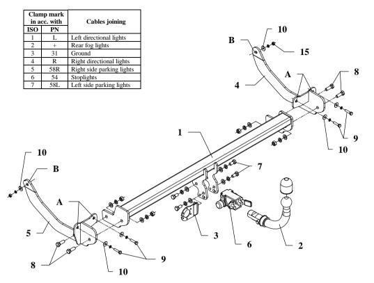
This towing hitch is designed to assembly in following cars: **PEUEOT 308SW (estate)**, produced since 2008, catalogue number **F33A** and is prepared to tow trailers max total weight **1700 kg** and max vertical mass **75 kg**.
