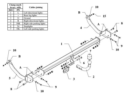
This towing hitch is designed to assembly in following cars: **PEUEOT 308SW (estate),** produced since 2008, catalogue number **F33** and is prepared to tow trailers max total weight **1700 kg** and max vertical mass **75 kg**.
