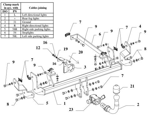
This towbar is designed to assembly in following cars: **Peugeot 807, Fiat Ulysse, Citroen C8, Lancia Z** (all 5 doors and VAN) produced since 2002 cat. no. **F26A** and is prepared to tow trailers max total weight **1850 kg** and max vertical load **76 kg**.
