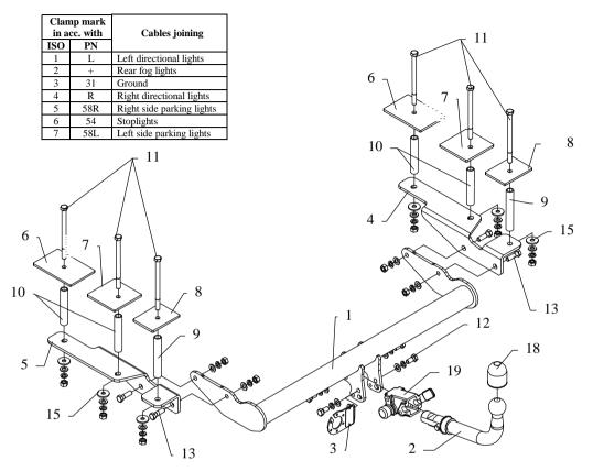
This towing hitch is designed to assembly in following cars: **OPEL VECTRA ESTATE**, produced since 2003 till 2008, catalogue number **E47A** and is prepared to tow trailers max total weight **2000 kg** and max vertical load **85 kg**.
