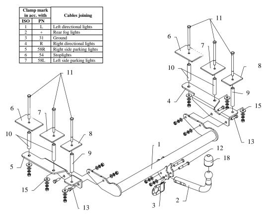
This towing hitch is designed to assembly in following car: **OPEL VECTRA ESTATE** produced since 2003 till 2008, catalogue number **E47** and is prepared to tow trailers max total weight **2000 kg** and max vertical load **85 kg**.
