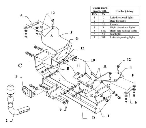
This towbar is designed to assembly in following cars: **ALFA ROMEO 147, 3/5 doors**, produced since 2000, catalogue no. **AL37** and is prepared to tow trailers max total weight **1300 kg** and max vertical load **60 kg**.
